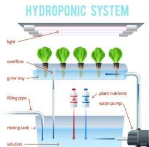
Fig 3: Dosing system overview
